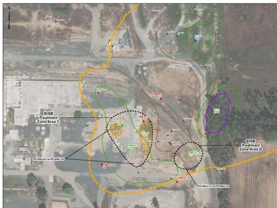
Figure 6 In-situ Bioremediation Substrate/Microbial Culture Injection
