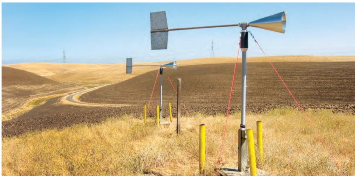
Figure 1 Wind-Driven Bioventing System
